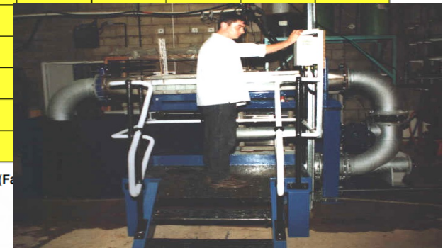
Figure 8.1 Measuring fish swimming speeds in a water tunnel (Fawley)
