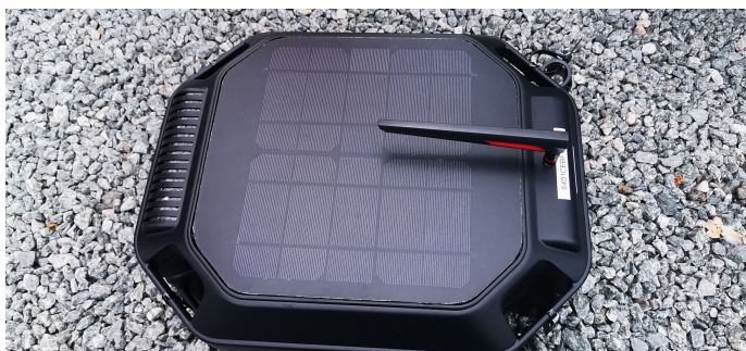
A WATR in-situ water quality monitoring unit
