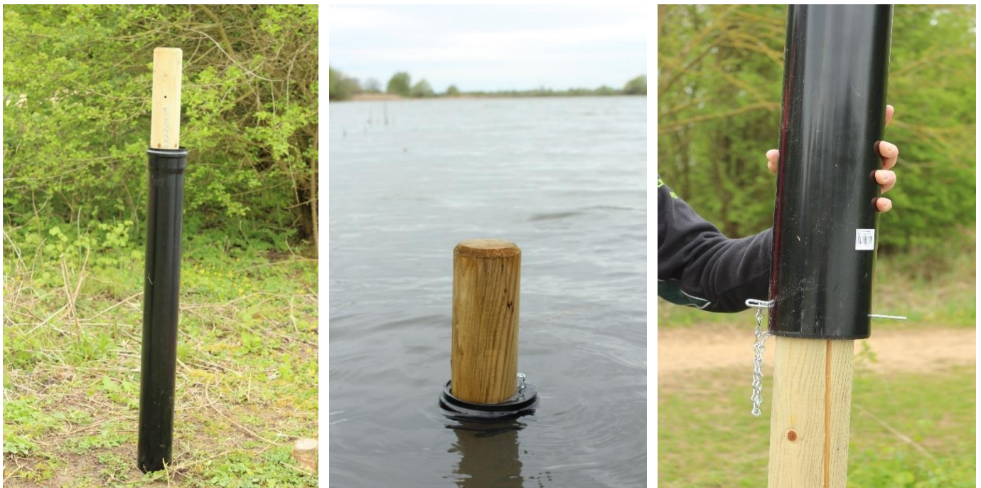
Lengths of black pipe supported by a wooden posts (left) and positioned in the margins of the fishery (middle). A peg inserted through the top (right) allows the pipe to be raised for drying.
